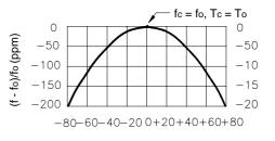
$\Delta T = Tc - To (^{\circ}C)$ The curve shown above accounts for resonator contribution only and does not include oscillator temperature characteristics.
