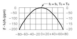
$\Delta T = Tc - To (°C)$ The curve shown above accounts for resonator contribution only and does not include oscillator temperature characteristics.
